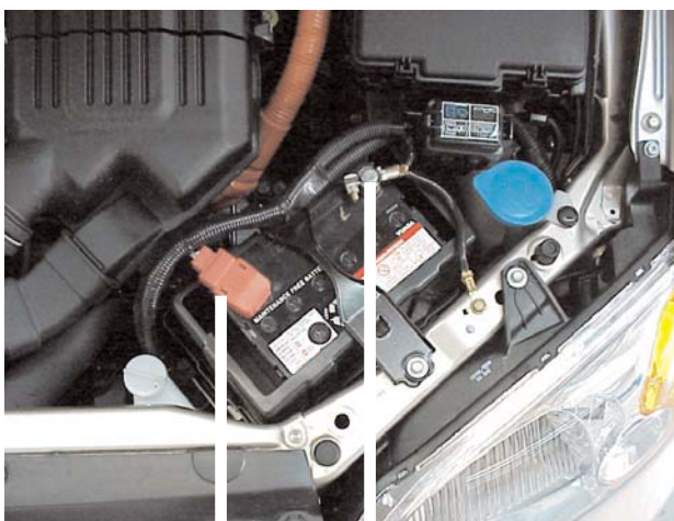
Positive Cable Negative Cable
