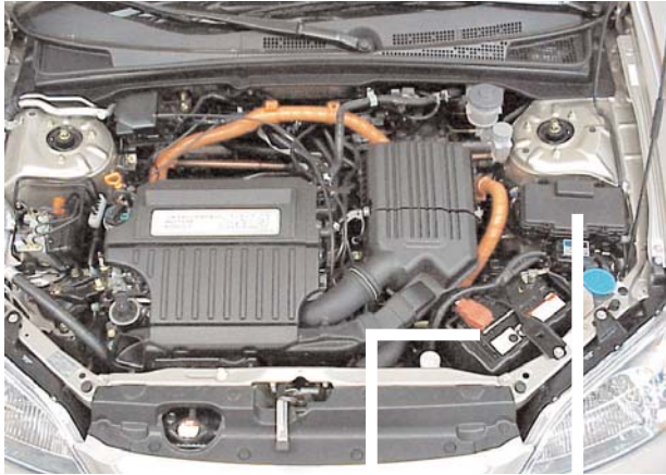
12 V Battery Under-hood Fuse Box
